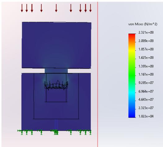
Figure 6: PTFE mold simulation with transitional fit clearance
