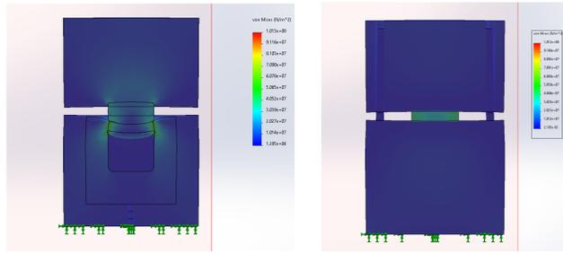
Figure 5: Deeper cavity simulation (left), Guide pin simulation (right)
