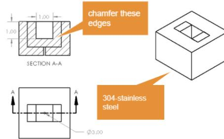
Figure 3: Preliminary PTFE mold design
