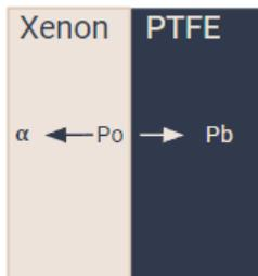
Figure 2: This figure shows one of two scenarios where a Po isotope alpha decays and the lead daughter nucleus goes into the wall and the alpha particle goes out into the detector.
