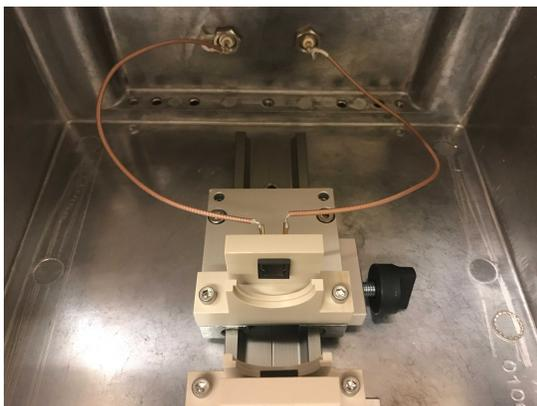
Figure 6: The image above shows the inner mechanism of the dark box as well as the photosensor.
