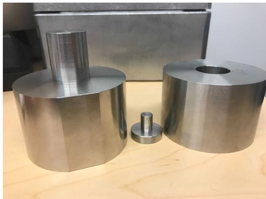
Figure 4: The image above shows the three manufactured components of the mold: the plunger (left), the plug (middle), and the body of the mold (right).
