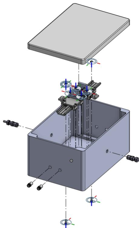
Figure 5: The image above shows an exploded view of the 3D model of the dark box design.
